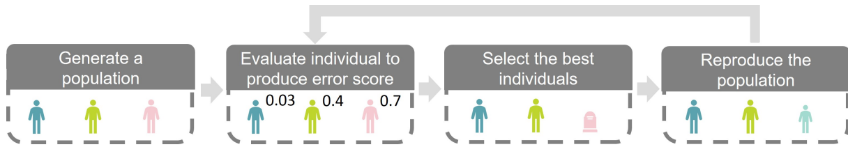
Figure 2.8: Evolutionary algorithm with the four main steps.
