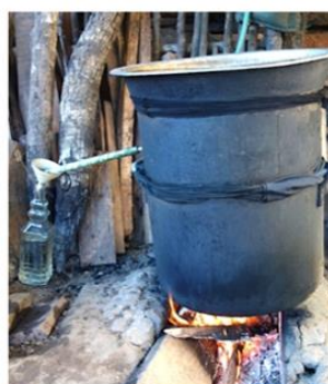
Figure 2. Traditional alcohol production device still in use in the Sayaboury province of Laos.
