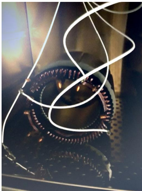
Figure 3-21 The stator in the oven’s chamber. The cables led to the outside that permit the measurements are visible.
