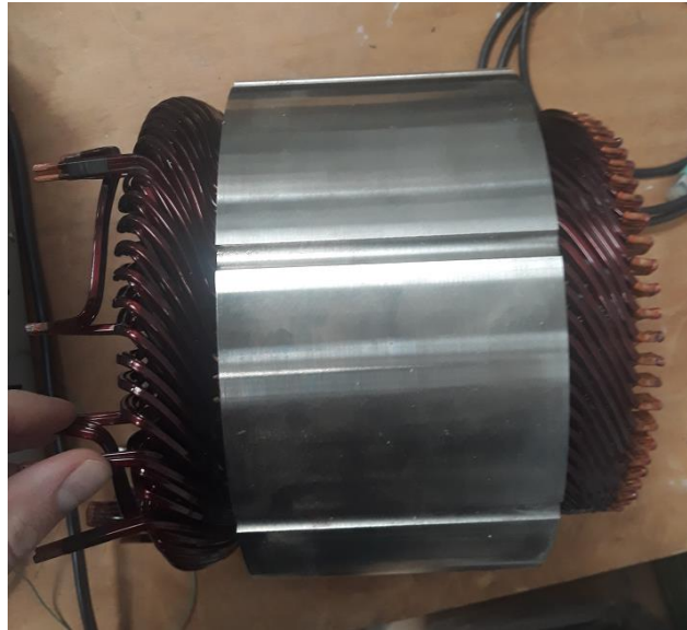
Figure 3-20 One of the two identical stator used in cycling tests.
