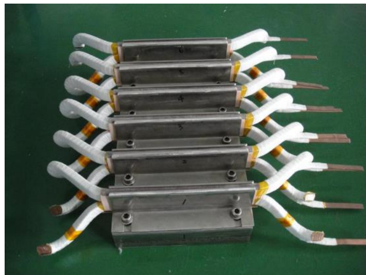
Figure 1-16 A formette for high-voltage form-wound machine qualification test [20].
