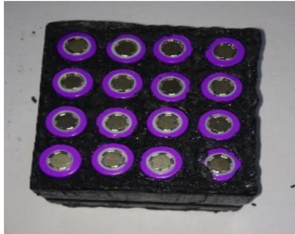
Figure I.19 Tested PCM cooling system with battery pack [78].
