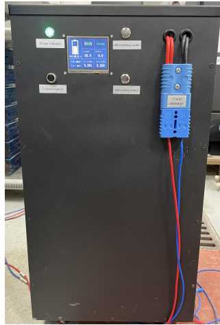
Figure 5.4 – LifePO4 lithium battery.
