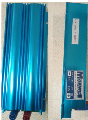
Figure 5.5 – Supercapacitor module (left) [161] and supercapacitor pack (right).
