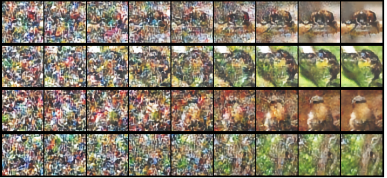
FIGURE 5.6 – Sampling denoising chain from t = 500 up to t = 0 , shown at regular intervals, conditioned on the outer part of the picture. We show only the last 500 steps of this process, as the first 500 steps are not visually informative. The sampling procedure is described in Appendix A.2.2.
