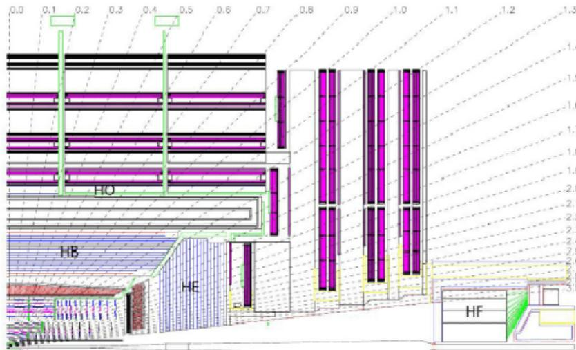
**Figure II.10** – Layout of a quadrant of the HCAL [48] and of its main structures: the barrel HCAL (HB), the endcap HCAL (HE), the outer HCAL (HO) and the forward HCAL (HF). The tracker system and ECAL are also illustrated in the bottom left corner.
