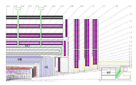
**Figure II.10** – Layout of a quadrant of the HCAL [48] and of its main structures: the barrel HCAL (HB), the endcap HCAL (HE), the outer HCAL (HO) and the forward HCAL (HF). The tracker system and ECAL are also illustrated in the bottom left corner.
