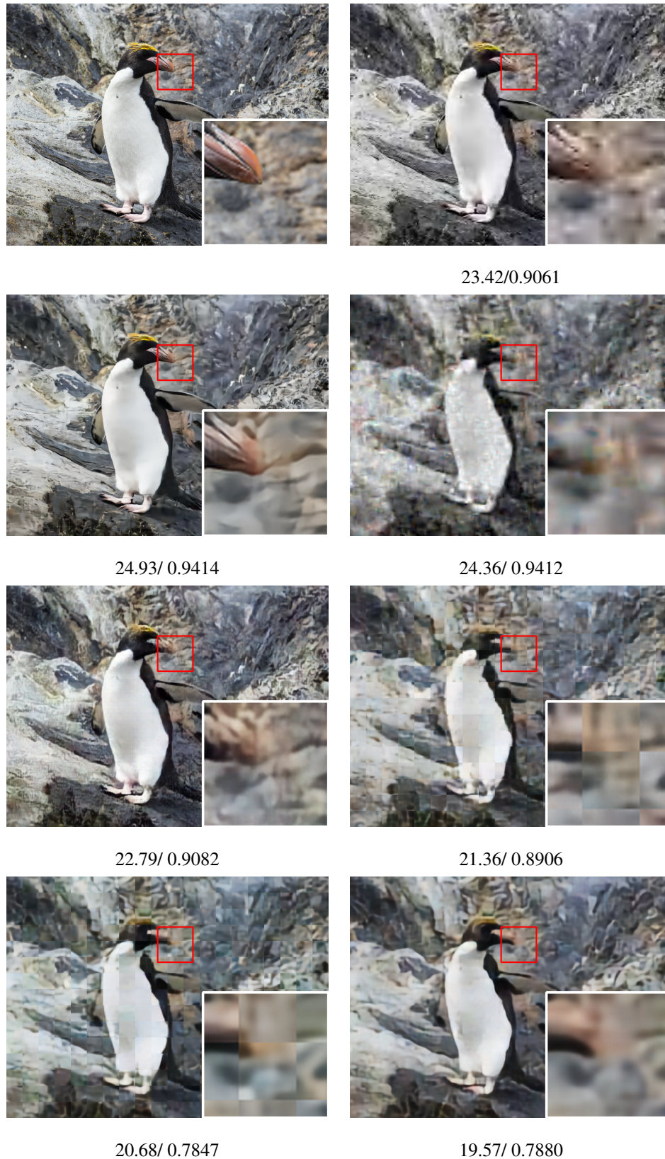
Figure 4.9: Image compression results at 0.25bpp on the test image indexed 801 of the DIV2K validation dataset. From top to bottom: Original image, JPEG2000, CAE-PSNR, WD-TV3D, CAE, our BBD, NQE- PI-PURENET and NQE- Full-Resolution PURENET along with the corresponding PSNR/ MS-SSIM values under each image.
