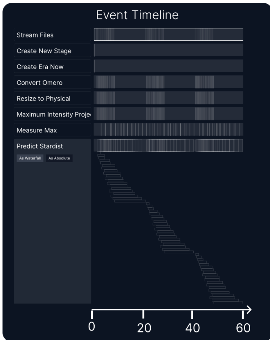
Figure 65 The Arkitekt Waterfall diagram, as inspectable on the WebUI inside Arkitekt, but trimmed for the first hour for clarity. The Predict Stardist node is unfolded showing all tasks, illustrating the processing time for each assigned task. The processing time corresponds from the time interval of assignment till the task is finished. As the node was parallelized 3fold, bars overlap, however as task length is still increasing, this node needs to be considered as bottleneck for the analysis, which is only compensated by the acquisition pause (processing could continue and catch up).
