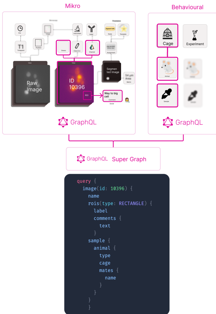
Figure 74 The GraphQL Supergraph with two different services (here Mikro and the fictional Behavioural service). Both services can stand and develop completely standalone but can be merged to a unified and inspectable service.
