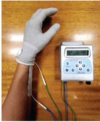
Figure 1 Electro-stimulation glove , plane electrode placed on the wrist and Micromed® stimulator set on 20 Hz; 1000ms; 800 \mu ; trig OUT, with variable intensity (mA) according to each subject's individual calibration
