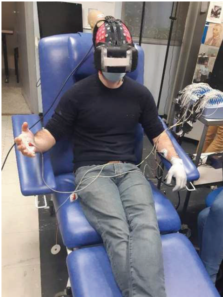
Figure 4 Example of subject installation – EEG recording cap, ECG and skin conductance electrodes; electro-stimulation glove; HTC Vive iVR glasses.
