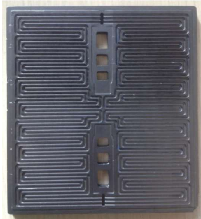
Figure 1.2.: Actual geometry form of cathode gas supply channel [83]
