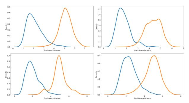
Figure 16: Activation vectors distances of the first 4 classes of CIFAR-10. The x-axis represents the Euclidean distance values, and the y-axis represents the distribution density (e.g., amount of points). The blue line represents the distance distribution between true positives, and the orange line represents the distance distribution between true positives against false negatives.
