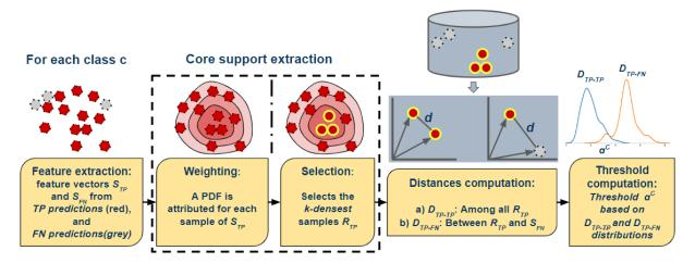
**Figure 15:** SENA monitor building. 1) A core support extraction algorithm is applied for weighting and selection of the most representative true positive neural activations to be stored and used at runtime. 2) It calculates the neural activation similarities among representative true positives, and also between true positives and false negatives.
