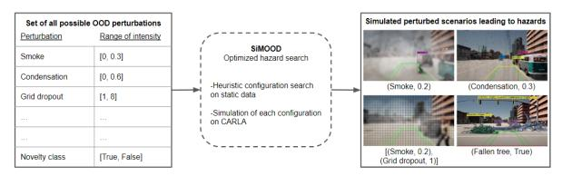
Figure 7: SiMOOD simulation flow. After an initial configuration of all possible perturbations, the algorithm searches possible candidates that will lead to hazards during simulation.
