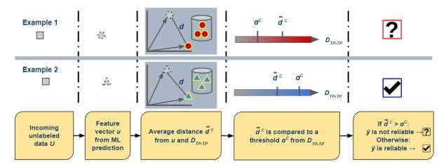
Figure 19: Two examples of SENA monitoring a class at runtime. The average distance  $\bar{d}^c$  is calculated by comparing the feature vector from the incoming image to  $D_{TP-TP}$  1) SENA triggers an alarm since  $\bar{d}^c > \alpha^c$  (unreliable prediction); 2) SENA does not interfere in the ML prediction since  $\bar{d}^c \leq \alpha^c$  (reliable prediction).
