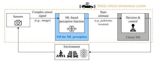
Figure 1: Safety Monitors for Machine Learning-based Perception Functions. In modern autonomous systems, state estimation provided by deep learning models cannot be trusted to make safety-critical decisions. Therefore, specific fault tolerance approaches should be implemented to ensure that failures of the ML perception function will not lead to catastrophic outcomes.
