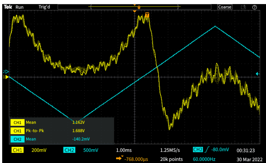
Figure A.3: MTS signal after optimisation on the PMC 16. The error signal presents some oscillations probably due to reflection at the splices of the fiber. The MTS signal presented here is filtered with a 1 kHz bandwidth after demodulation.
