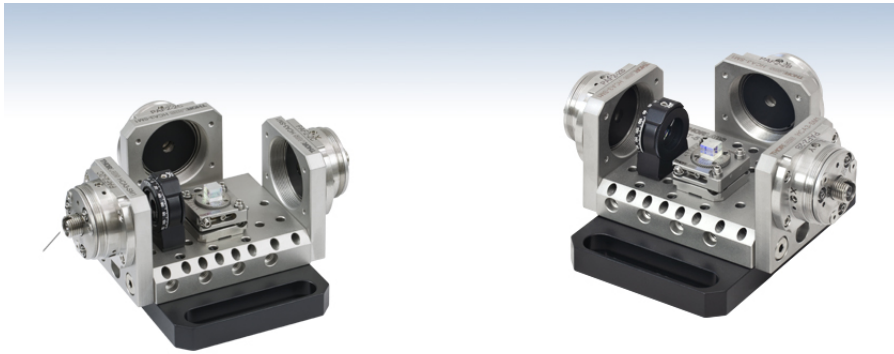
Figure 3.16: Compact free space bench for injection of the fiber. Connecting both side of the fiber using butt coupling did not yield a exploitable MTS signal. One side of the fiber had to be injected in free space.
