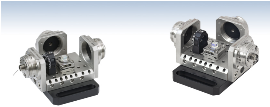
Figure 3.16: Compact free space bench for injection of the fiber. Connecting both side of the fiber using butt coupling did not yield a exploitable MTS signal. One side of the fiber had to be injected in free space.
