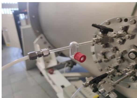
Figure II.18: The impinger used to inject liquid VOCs into CHARME.
