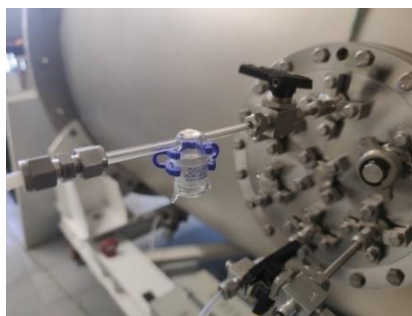
Figure II.19: The impinger used to inject solid VOCs into CHARME.
