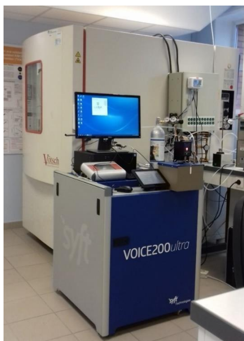
Figure II.12: A picture of the THALAMOS-ASC connected to one of the analytical techniques, SIFT-MS (Voice200).
