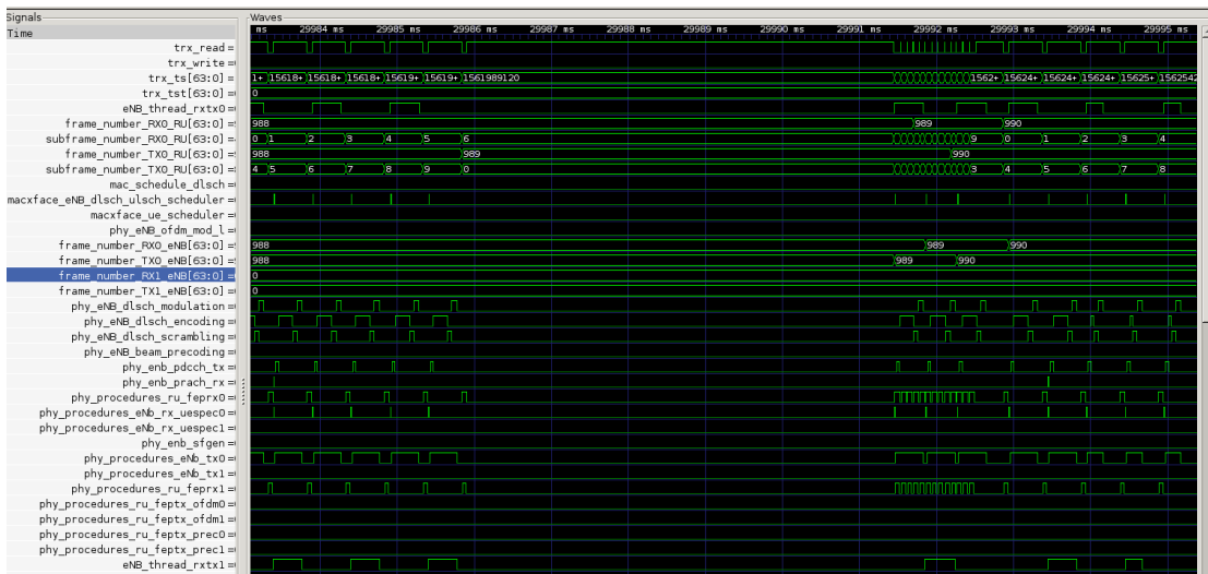
Figure 5.8 – The timing log of the recovery of the pipeline structure
