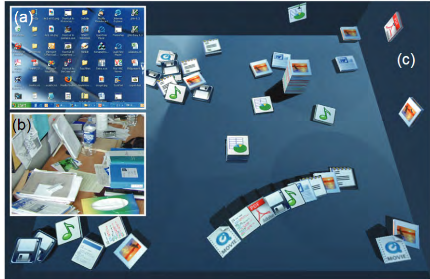
Figure 2.12: (a) Traditional virtual desktop layout with organised content. (b) A physical desk where items are arranged in a casual manner. (c) The BumpTop prototype uses piles to organise content and uses a physics simulation to allow for more natural and authentic interaction for a more realistic experience [Agarawala and Balakrishnan, 2006]
