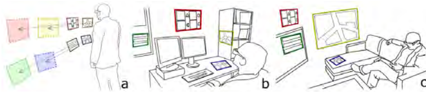
Figure 2.21: Example of spatial consistency constraint: The transition of the virtual content from a body-centric layout to world-fixed coordinates (a). The spatial relationships between the elements are preserved while moving from one environment to another (b,c). [Ens et al., 2015]
