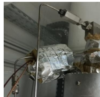
Figure II.6: Detail of preheater installed in calcium line
