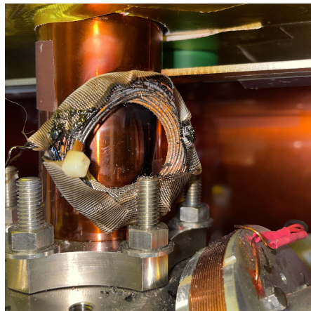
FIGURE III.37: The state of the Stern-Gerlach when the magnetic-shield are opened.
