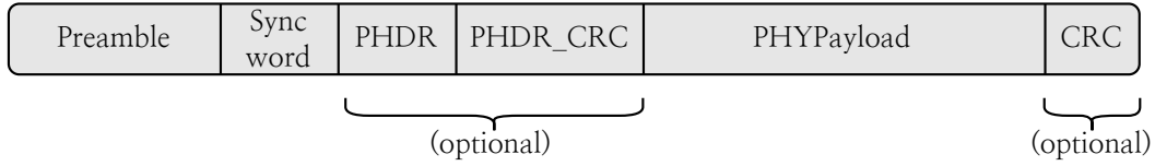
Figure 1.3: LoRa physical frame structure
