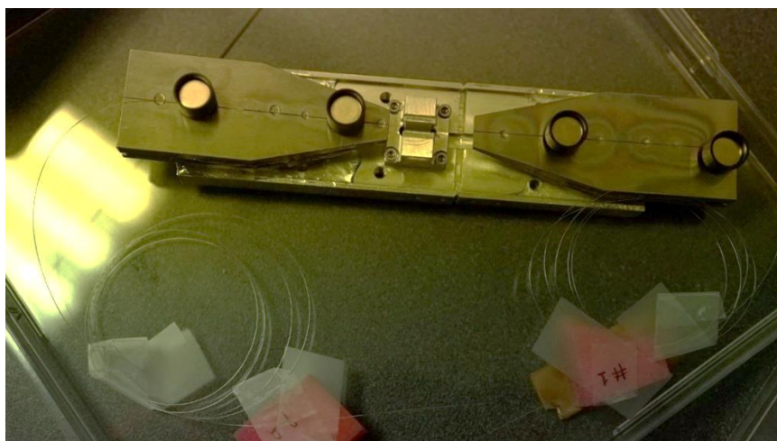
Figure III-46: The ultimate result of the manufactured device for the 5-pass waveguide after connectorization with radiation hardened fibers for the perspective of in-situ radiophotoluminescence and radiation-induced attenuation.
