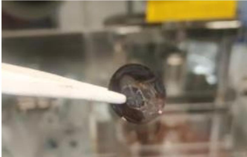
*Image of a graphite electrode in its delithiated state after experiencing 500 cycles in the range of 2.5 to 4.3 V at 1C in graphite/NMC811 cell (25°C). Prior to capturing the photograph, the electrode was rinsed with DMC. The presence of grey and golden spots on the graphite surface advocates for the presence of metallic lithium deposits.*
