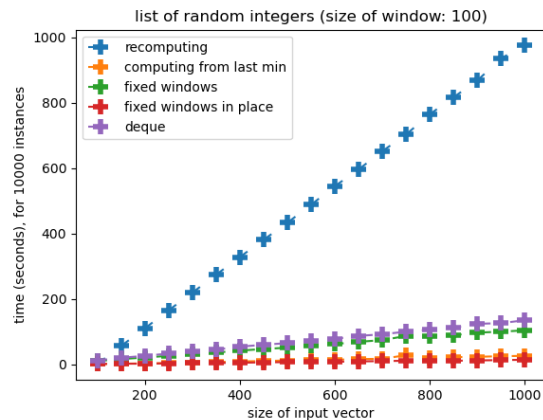
Figure 4.7: Comparison between 5 approaches for computing sliding window minimum. The input vector is composed of random integers. The size of the window is set to 100.
