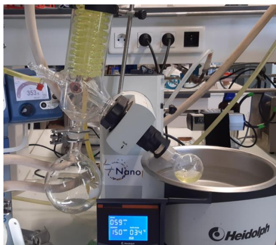
Fig. 2: solvent evaporation during the synthesis of PLSH.
