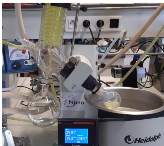
Fig. 2: solvent evaporation during the synthesis of PLSH.
