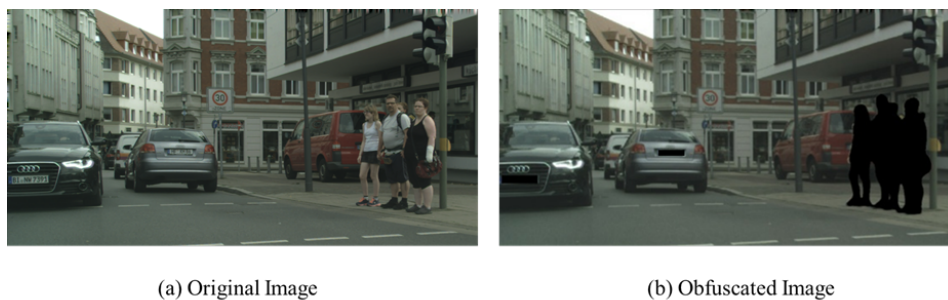
Figure 3.5: Obfuscating the license plates and the individuals on the street. Image taken from the cityscape dataset [Cordts et al., 2016]
