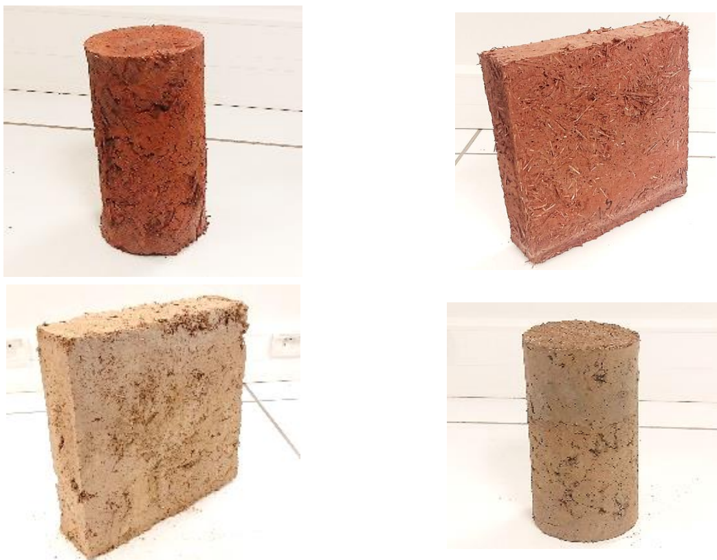
Figure 3.6 Coffee lightened clay and Structural cob samples used for mechanical ( \text{Ø}11 \text{ cm} \times 22 \text{ cm} ) and thermal ( 30 \times 30 \times 4 \text{ cm} ) tests [165]
