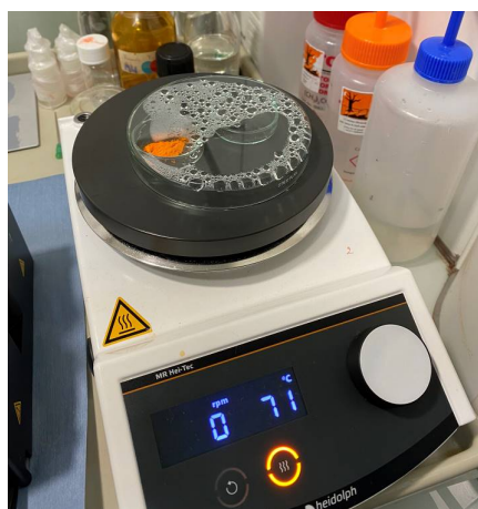
Figure 4-1-3. Humidified \text{MAPbBr}_3 SC powder for evaluation of water incorporation during ATR-FTIR analysis.
