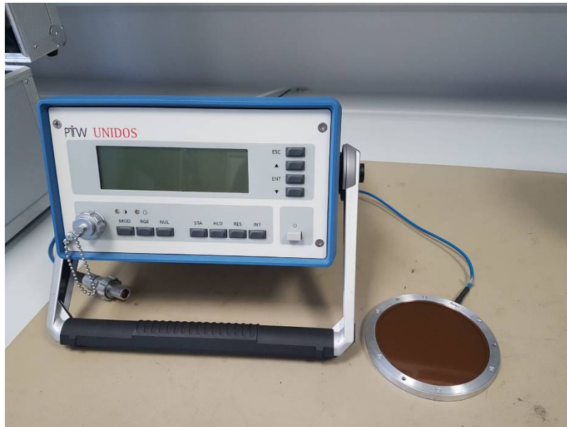
Figure 2-3-3. PTW UNIDOS dosimeter used to calibrate the X-ray dose delivered by the tube in atmospheric conditions.
