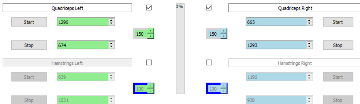
Figure 5.3: Snapshot image of the designed graphical user interface (GUI) for the stimulation parameter setup. Four muscles along with the maximum stimulation intensities (in mA) can be selected. Start and stop positions for each muscle can be chosen by placing the leg in the position and clicking the adjacent “Start” or “Stop” button. The horizontal bar in the middle represents the stimulation intensity applied to the muscles as a percentage of the selected maximum stimulation intensity.
