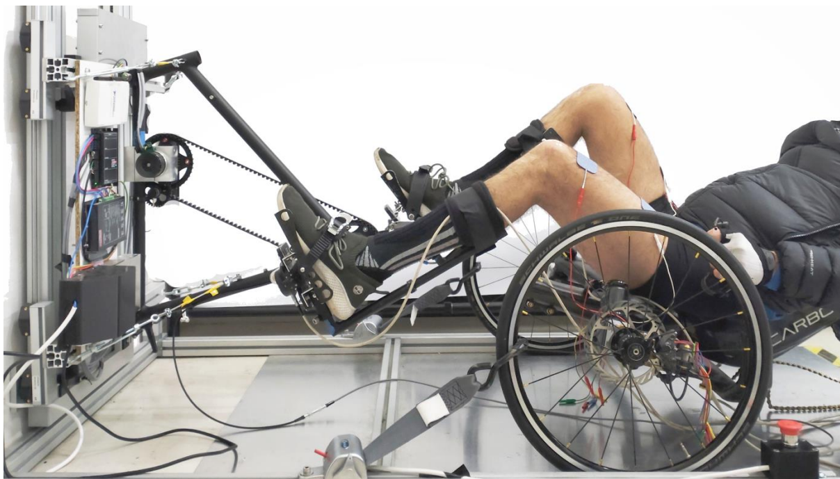
Figure 2.3: Photo of an SCI subject using the platform from the Carbontrike.
