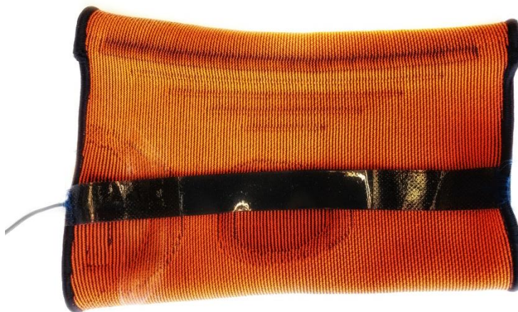
Figure 5.1: A photograph of a stretch sensor sewn into a knee brace.
