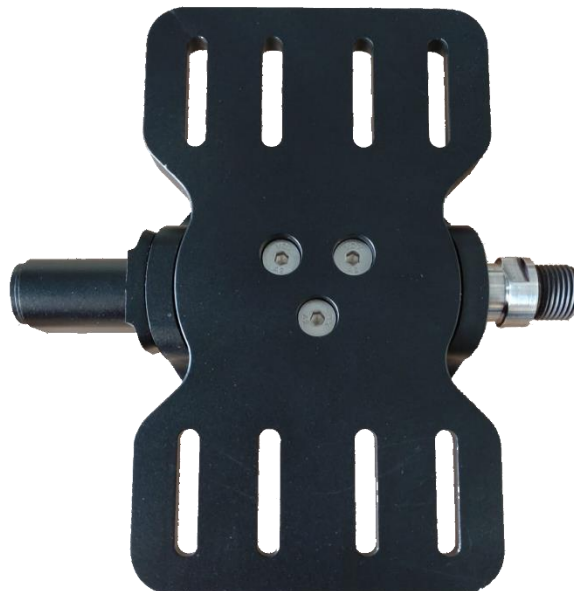
Figure 2.2: A custom connecting plate attached to the force/torque measuring pedal.
