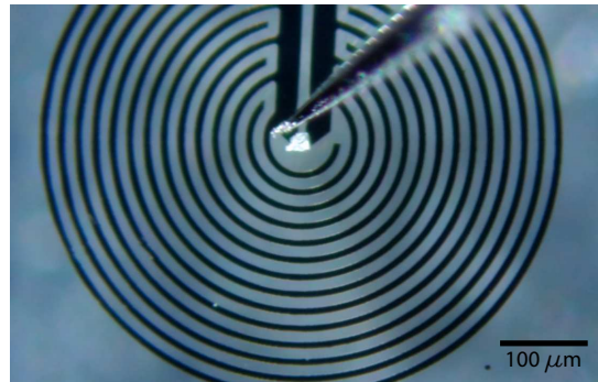
(b) Polypropylene piece being pushed into place using a tungsten tip.
