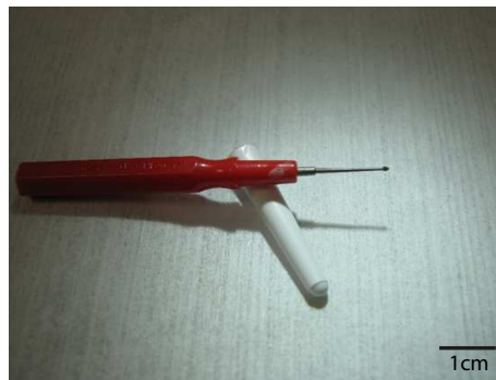
(b) Spatula used for the BDPA placements in Figure 3.21a.
