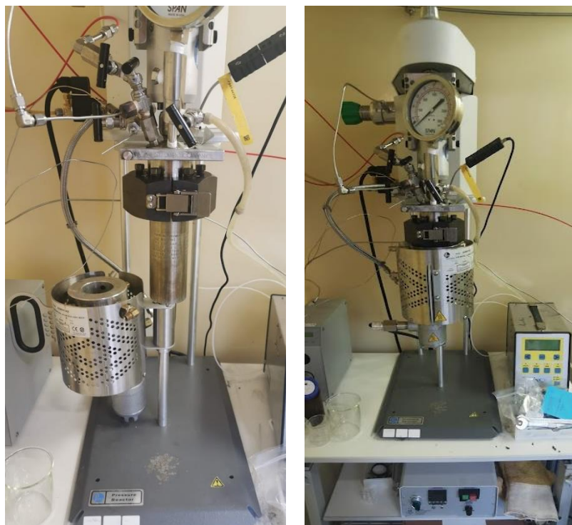
Figure 2-3: PARR reactor set-up for the non-radioactive hydrogenation of CNA.
