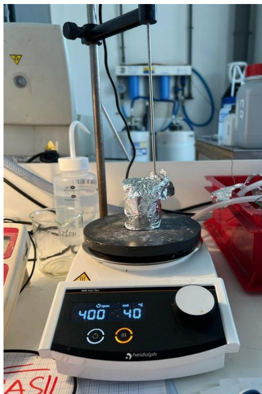
Figure 2-6: General set-up for azo-dyes decolorization.
