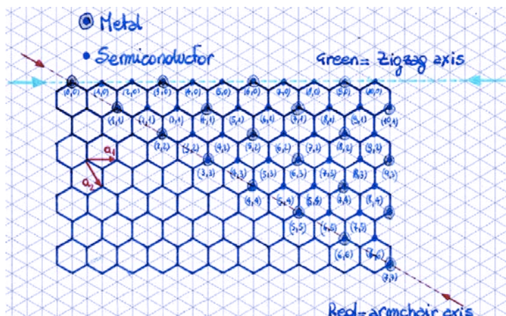
Fig 5.4 The conventional structure for a carbon sheet of a nanotube Source: AD
