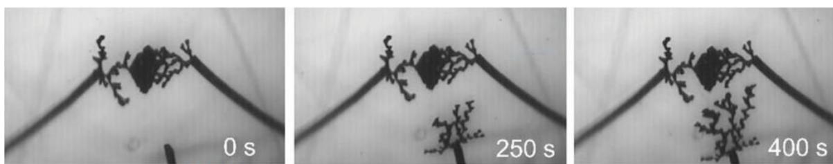
Figure 20. Time-lapse of a third dendrite formation using the AC electropolymerization process at 5 V p , f = 80 Hz, 50% dc and 0 V off while earliest dendrites are set as ground 9 .
