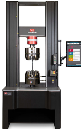
Figure 2-4 : Le banc de traction Instron 68FM-100.
