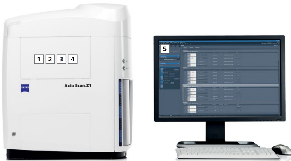
Figure 1.11: Left: Axio Scan Z.1 and right: image viewing software Zen. 1. Microscope, 2. objectives, 3. illumination, 4. cameras and 5. software.
