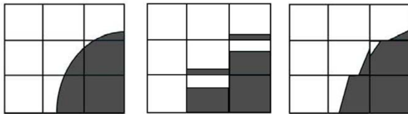
Figure 2.5: Application of VOF method, where dark is liquid and white is gas. Left : initial flow field. Middle : transported \alpha_l field. Right : interface reconstruction, where a non-smooth interface can be appreciated. Source: Odier (2006)
