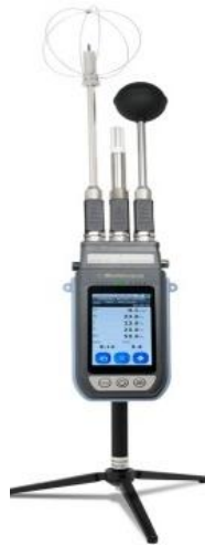
Figure 13: Delta Ohm HD32.3TC captured indoor micro-climate
