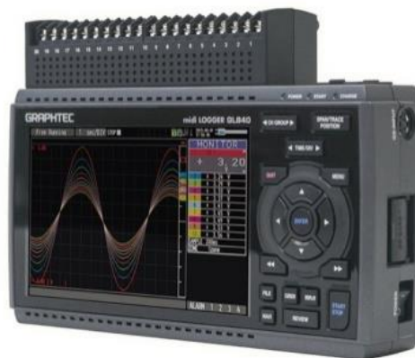
Figure 14: Graphtec GL840 captured the surface temperatures
