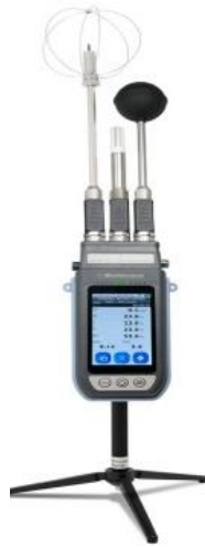
Figure 13: Delta Ohm HD32.3TC captured indoor micro-climate
