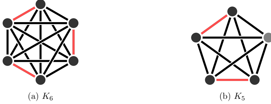
Figure 9 – Perfect matching ■ for complete graphs K_N , with even N . For K_N with odd N , some vertices are not matched ■ .
