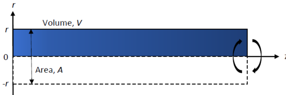
Figure 4.3: Diagram of the cylindrical integration along the z-axis in a 2D axisymmetric model
