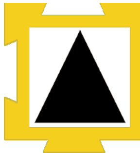
Figure 4.13: The detection triangle is on the back of upper-left side of the prototype. This stark contrast and simple geometry have been specifically chosen to ease detection.
