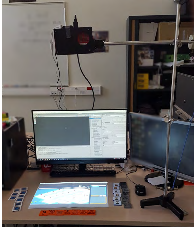
Figure 4.2: Third prototype being tested in the laboratory. Some of the tokens can be seen around the projected area on the bottom. The chemistry lab equipment that was used to hold the project is on the right. On the top of the image are the projector with the webcam behind it filming the game are below.
