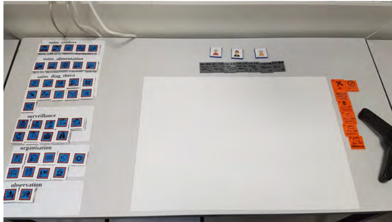
Figure 4.16: Table with the tokens' placement around the main interface that is projected on the blank paper at the centre. The paper is used to maximise light reflection as a projector can be lacking in light intensity. Using it helps keep the conditions similar across test sites.
