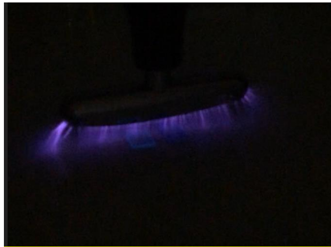
Figure 3.5 – Plasma activation of DF layers for bonding. Following the plasma treatment, the surface of the material is rich in polar molecules. UV radiation and active oxygen species generated by the plasma disintegrate separating agents, silicones, and oils on the surface. The vacuum system efficiently removes these byproducts. Concurrently, the active oxygen species, or radicals, in the plasma, adhere to active surface sites across the material, resulting in a highly receptive surface for bonding agents.
