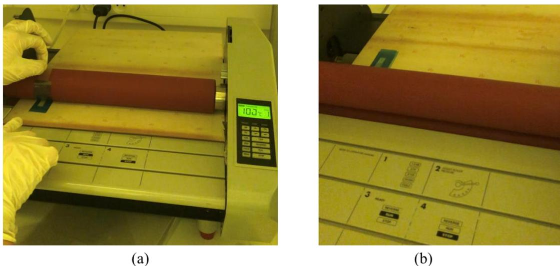
Figure 3.4 – Lamination of a DF layer onto a PMMA substrate.
