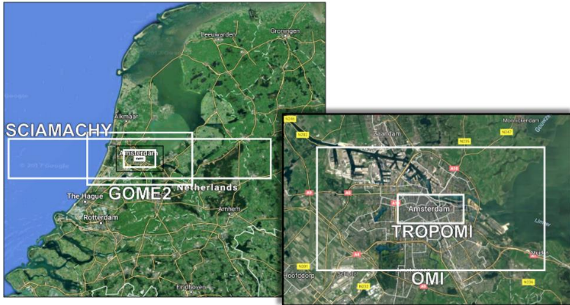
Figure 26 Spatial resolution comparison of satellite instruments. Note that TROPOMI pixel size further decreased now (Taken from BIRA-IASB, www.aeronomie.be/en/news/2021/three-years-tropomi-measurements )
