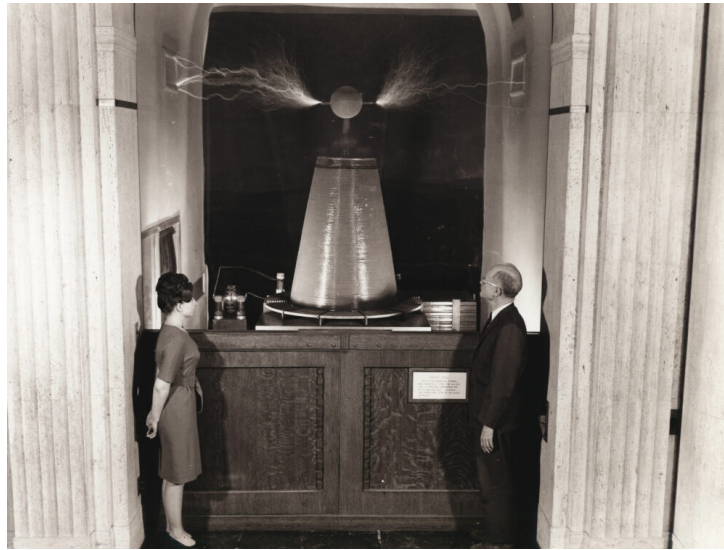
FIGURE 4.1 – Bobine de Tesla ( https://griffithobservatory.org/exhibits/ ).
